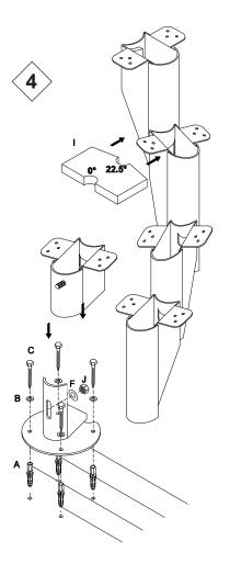
Mount the steps using torx-spax screws (K) and the enclosed bit (A1).
