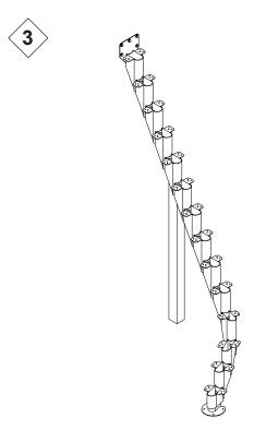
For quarter-newelled staircases, turn the 3 last middle elements and the bottom element 22.5°, using the enclosed assembly piece (I). The 5 first steps should then face the same way. If you shoose this staircase design, care must be taken when using the staircase.
